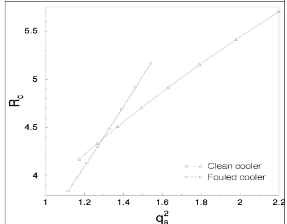
Shift of the surge limit line due to variation in intercooling. The compressor which surges first changes with the fouling of the cooler
