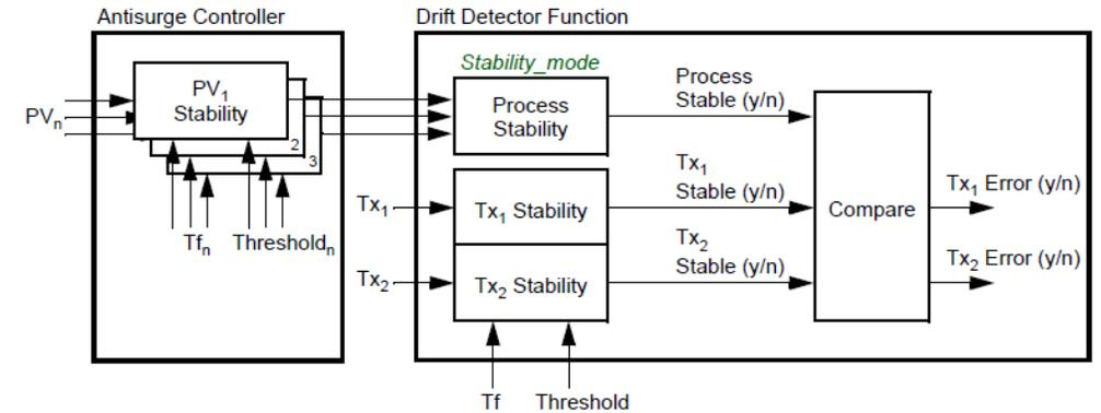
Figure 1-1 Drift Detector Function Overview
