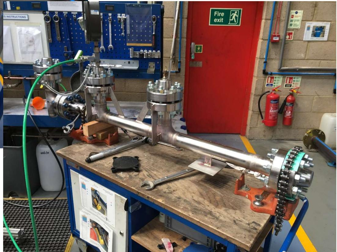
Tested at 721 barg and passed with flying colours, contains a vented float to allow it to function and is the highest rated unit we have ever manufactured. Our PED has been increased to accommodate this design.
