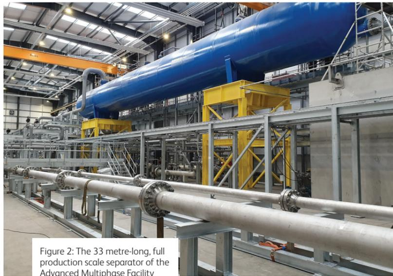
Figure 2: The 33 metre-long, full production scale separator of the Advanced Multiphase Facility
