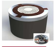
Design concepts for commercial Kibble balances. The balances would use electromagnetically generated force compensation and could measure masses from tens of milligrams up to a few hundred grams.
