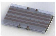
Electrostatic micro-Kibble balance concept for mass measurement from a few milligrams down to picograms
