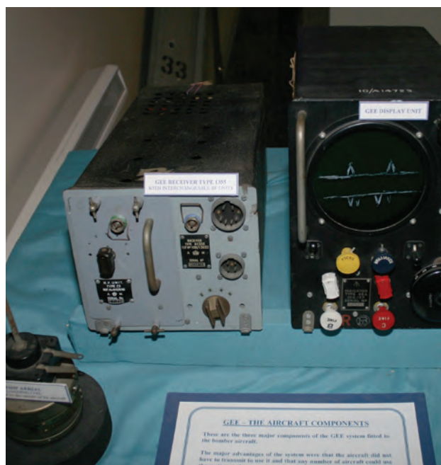
Gee Airborne Equipment at RAF Air Defence Museum. Picture credit: Jmb at en.wikipedia ( https://commons.wikimedia.org/wiki/File:J_M_Briscoe24_07_200713_05_14IMG2104_GEE_AIRBORNE.JPG ) https://creativecommons.org/licenses/by-sa/3.0/legalcode
