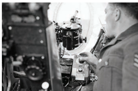
Image: IWM (CH 10853) A ground crew sergeant demonstrates the operation of the photo-reconnaissance camera in a De Havilland Mosquito of No. 540 Squadron RAF at Benson, Oxfordshire, using the Type 35 remote control box in the navigator's position in the nose of the aircraft.
