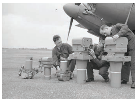
Image: IWM (CH 18399) Instrument workers line up aerial cameras at Benson, Oxfordshire, before installing them in a De Havilland Mosquito PR Mark IX: (left to right) two Type F.24 (14-inch lens) vertical cameras, one F.24 (14-inch lens) oblique camera, two Type F.52 (36-inch lens) 'split pair' vertical cameras.
