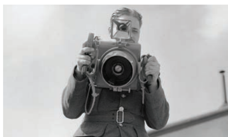
Image: IWM (CH 1247) A trainee air observer points a Type F.24 aerial camera at the PRU photographer. When operated by hand, the Type 21 mounting with hand grips and an eye piece was fitted, as seen here.
