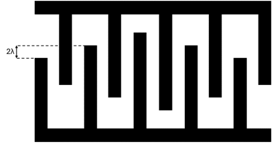
Figure 4. Apodized IDT configuration.
