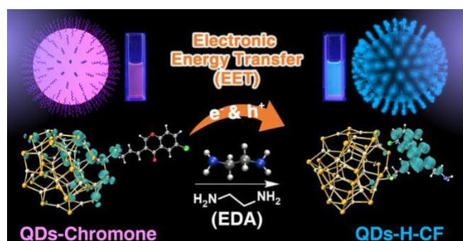
Figure 3. Schematic illustration of design strategy for colorimetric and fluorescent dual mode sensing materials by EET mechanism.
