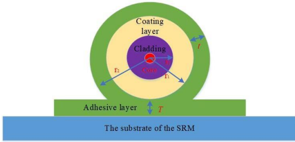
Figure 2. Coupling Model of Fiber Optic Sensor and SRM Matrix
