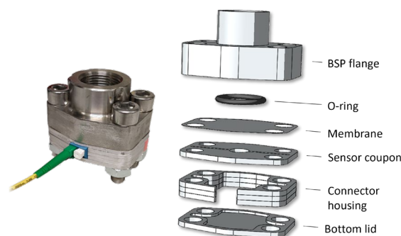
Figure 2. Schematic diagram of the sensor assembly and photograph of the fully assembled sensor. The sensing fibre and diaphragm are sandwiched between a flange and the connector housing, which holds the terminated fibres.
