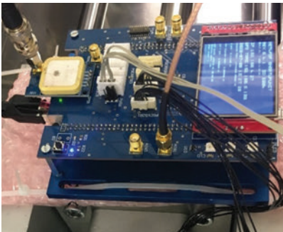
Figure 1: Smart up unit for the upgrade of existing measurement infrastructure with calibrated MEMS sensors and time stamps traceable to SI
