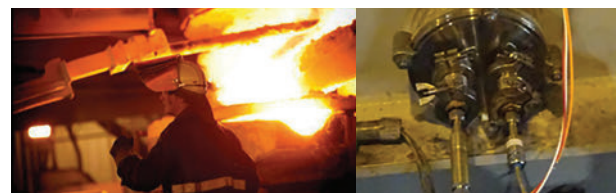
Figure 3: Left: Silicon processing environment. Right: Probes emerging from the space above the melt pool.
