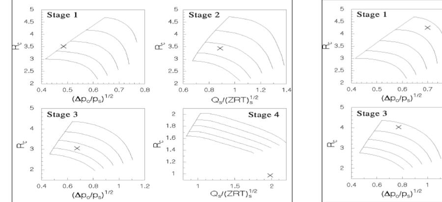
Operating at moderate to low speeds, the 4<sup>th</sup> Section may choke while the 1<sup>st</sup> Section surges.
