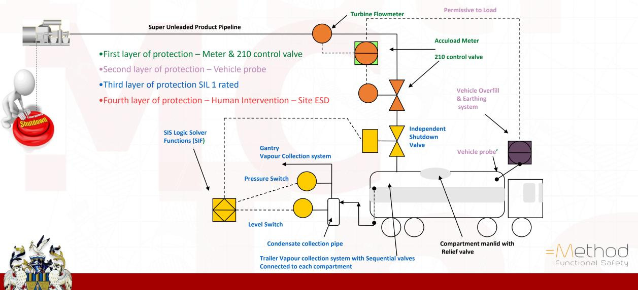
First Layer of Protection: Basic Process Control System
