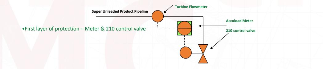
The product flow is regulated via a "210" control valve. This valve is controlled via the "Accuload" intelligent meter connected to the Terminal automation system. Post incident the 210 valve was tested and an intermittent fault discovered. The valve sticking in the open position was determined to be the immediate cause of the incident.
