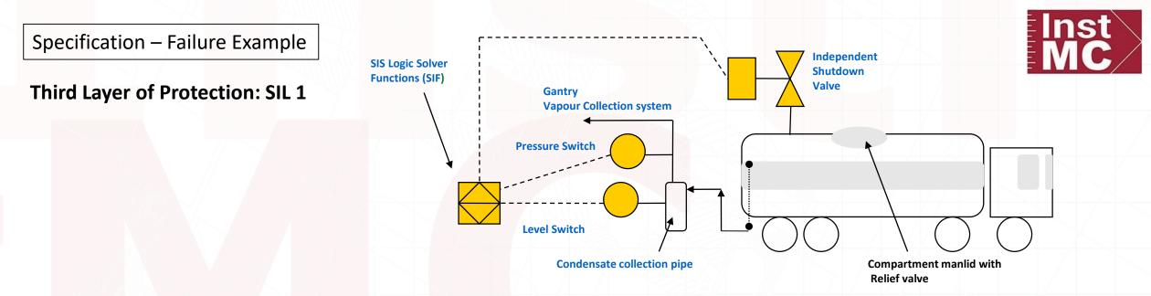
The design of the 3<sup>rd</sup> layer of protection is based upon product overfilling the vehicle compartment into the vapour recovery system and triggering a high level switch installed in a liquid collection pipe on the loading gantry. In addition a pressure switch detects a high pressure in the same vapour line.
