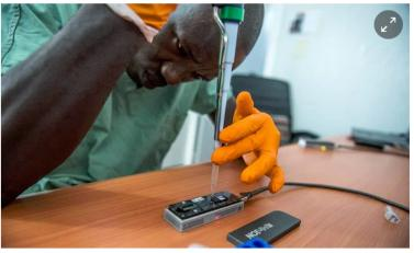
The MinION device, which weighs less than 100g, takes frequent electrical current measurements as a single strand of DNA passes through one of 2,000 pores in a plastic membrane. Photograph: Tommy Trenchard/EMLabs
